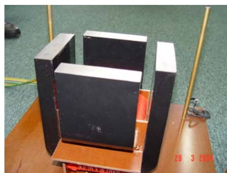
Fig.8. The design and construction of the 2D magnetising system (only the bottom part is shown)
